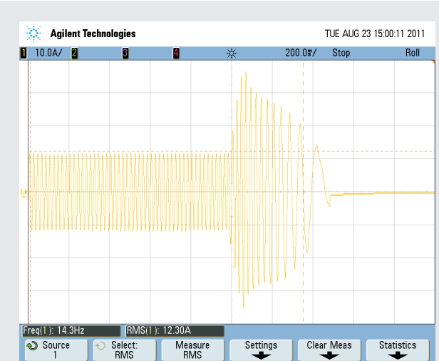
Flux braking current waveform in sensorless vector control mode with 50Hz (deceleration time: 0.5s)
